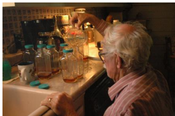
Fig. 4. Pouring agar solution in bottles prior to cooking, using a pre-measured upright bottle as a guide. Photo: DSC_7474 Thur-03 Dec-15.
