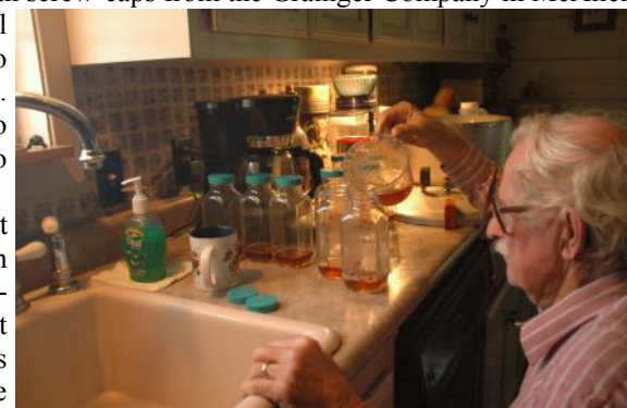
Fig. 3. Pouring agar solution in bottles prior to pressure cooking Photo: DSC_7473 Thur-03 Dec-15.
